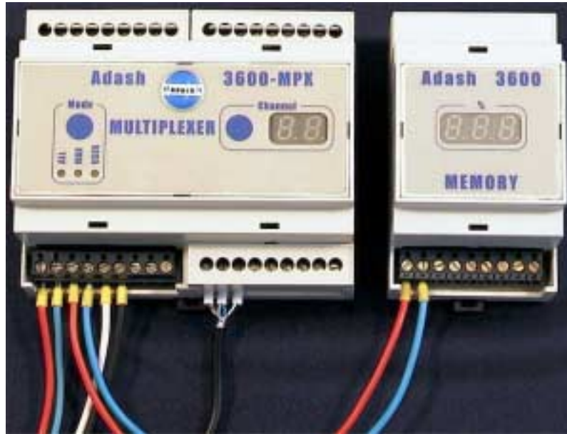
Fig. Interconnection of supply conductors
