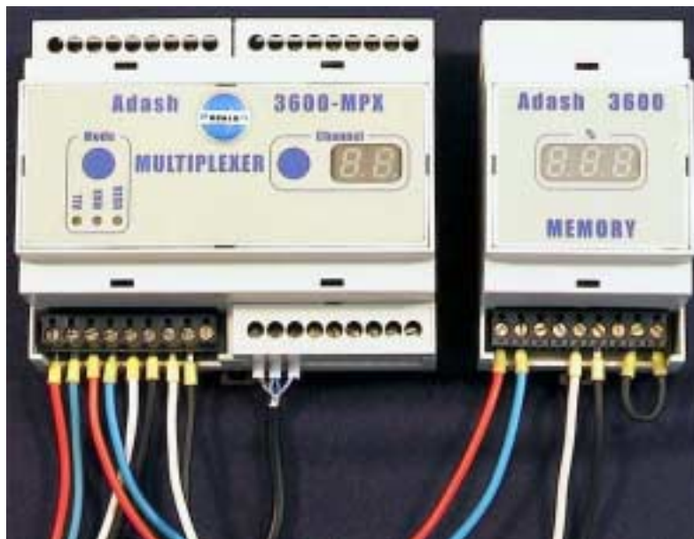
Fig. Interconnection of communication conductors
