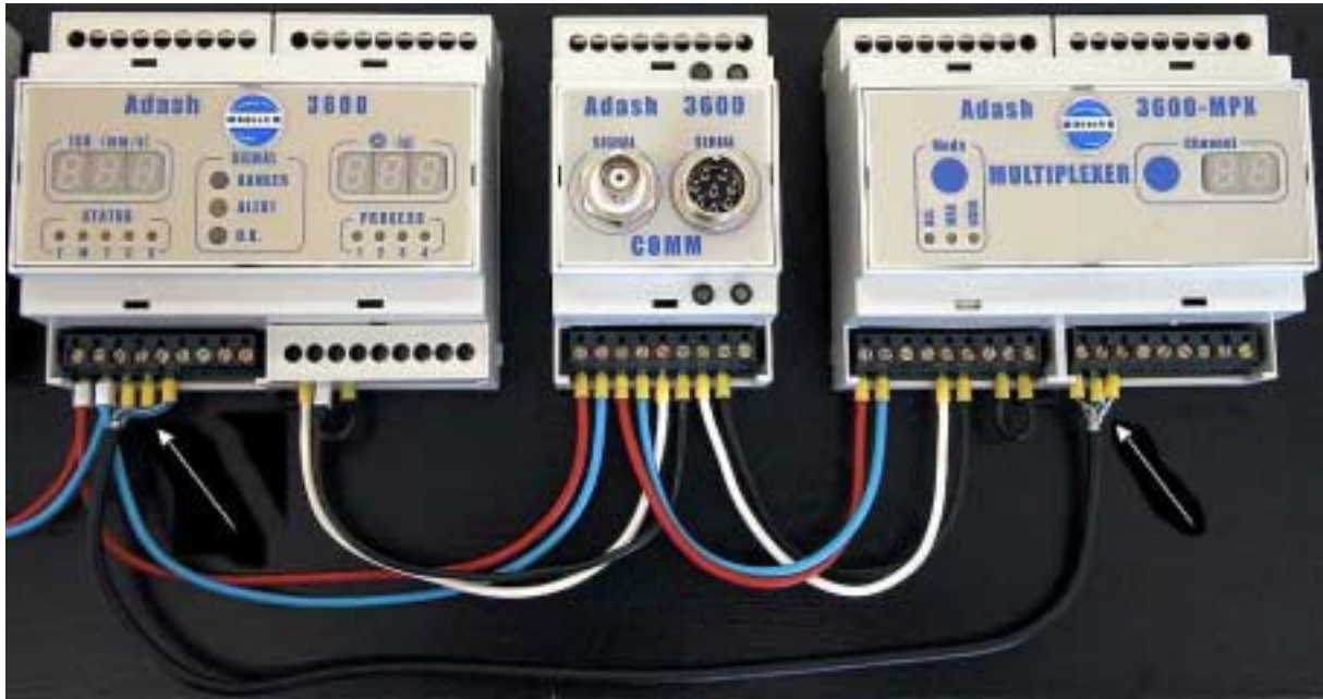
Fig. Interconnection of signal terminal connectors of the 3600-MAIN and 3600-MPX modules
