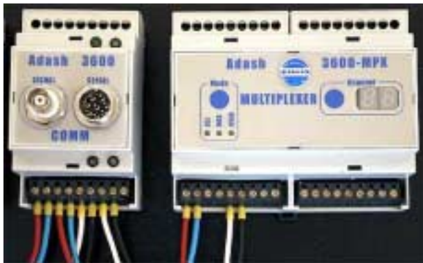
Fig. Interconnection of communication conductors
