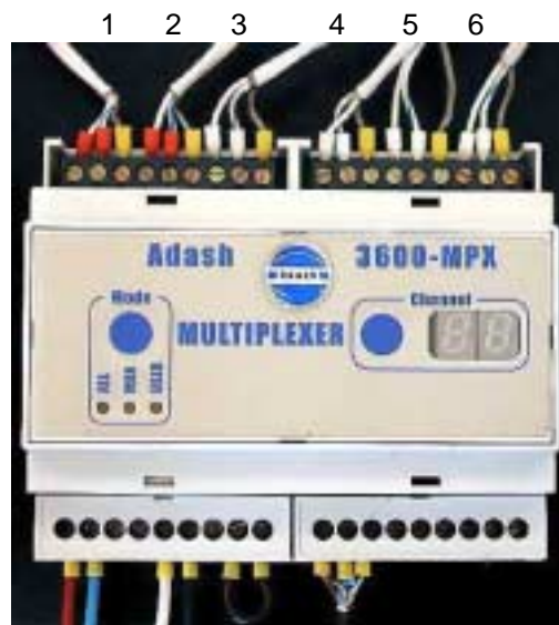
Fig. Connection of channels 1 - 6
