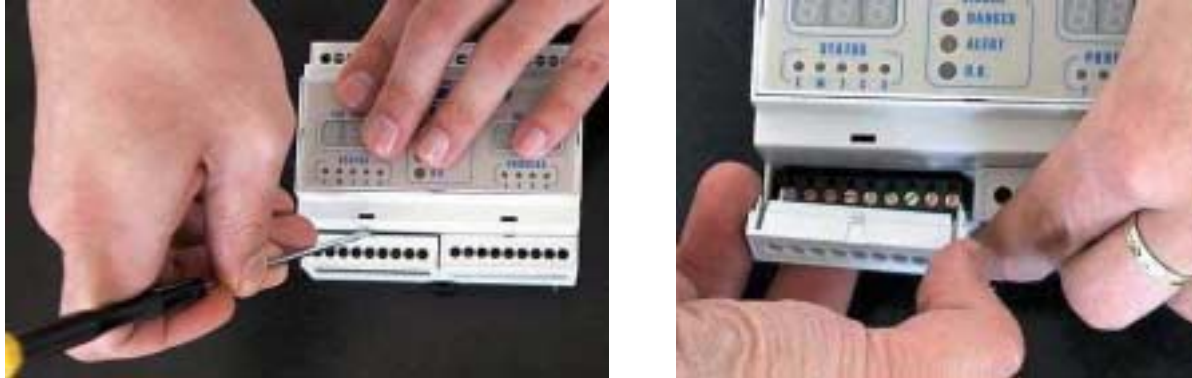
Fig. Removal of the terminal connector covers
