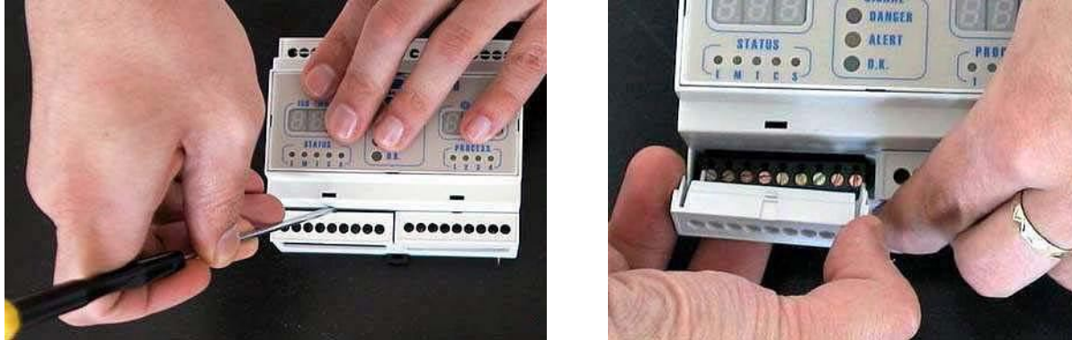
Fig. Removal of the terminal connector covers
