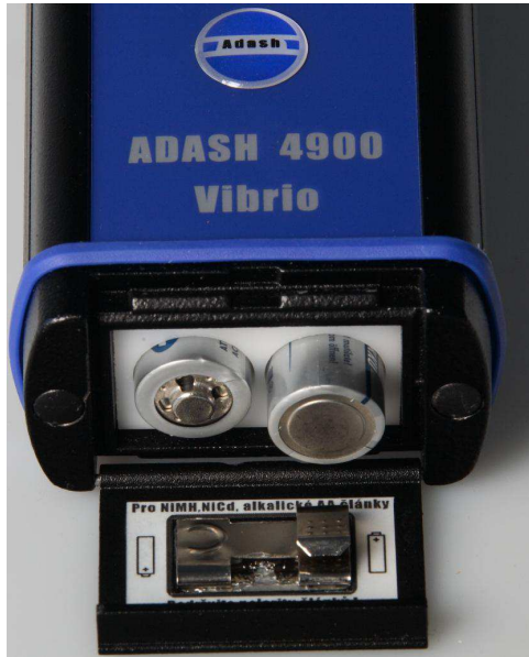
Fig. Placement of power batteries
